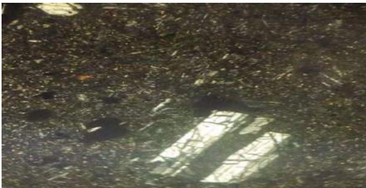
Figure 6.4. Microphotograph showing euhedral plagioclase feldspar porphyry in fine groundmass (Image under Cross Polar and 5X magnification).
