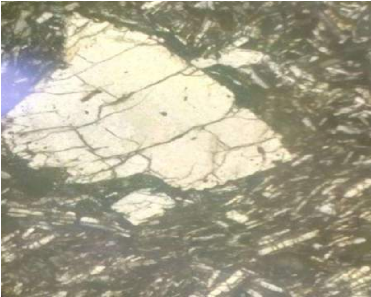
Figure 6.7. Microphotograph showing alkali - feldspar (Sanidine) phenocryst surrounded by fine groundmass (under Cross Polarize Microscope - XPL and magnification of 5X).
