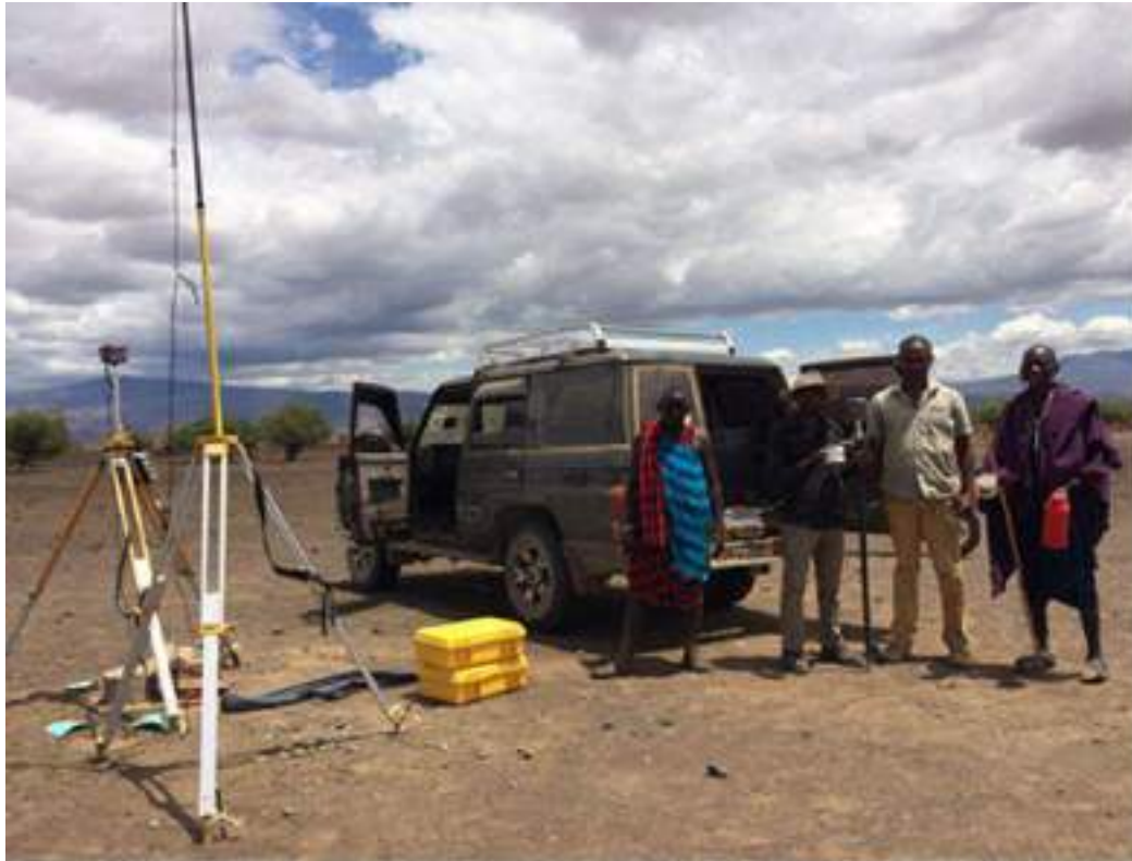
Figure 6.23. Photo showing DGPS base station with receiver and rover
