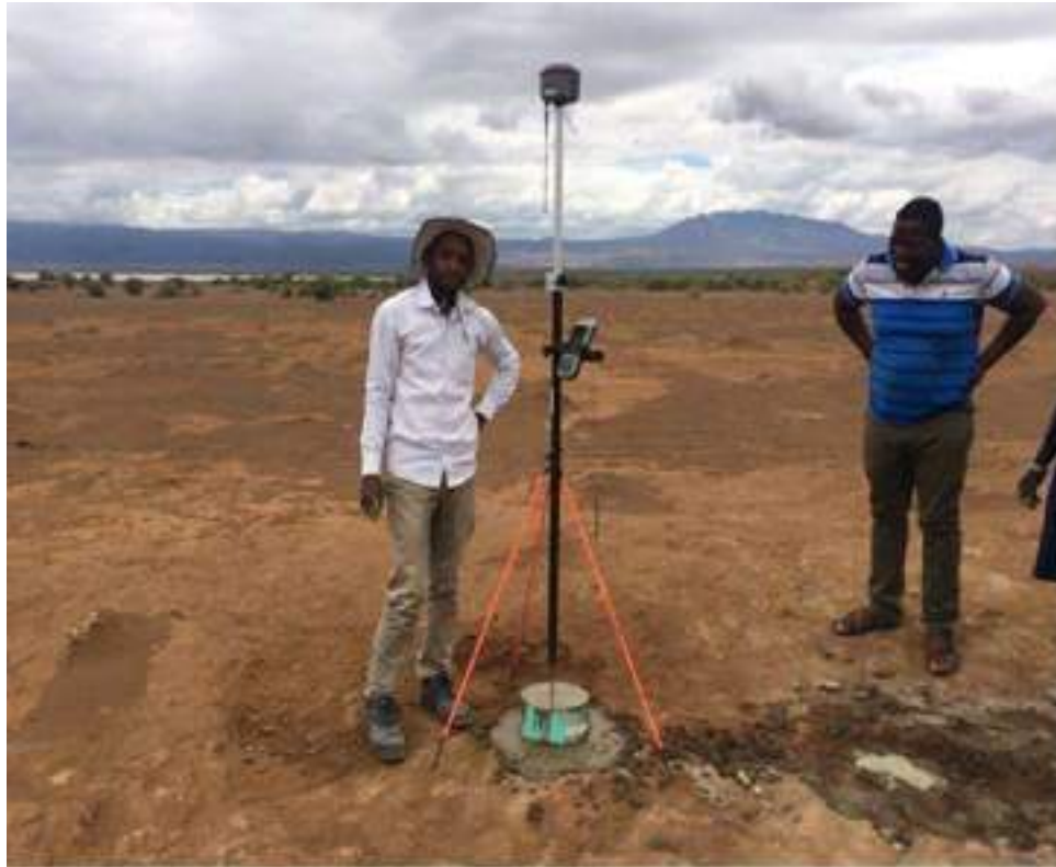
Figure 6.20. Photo showing DPGS positioned on the control points to record coordinate using RTK technique.
