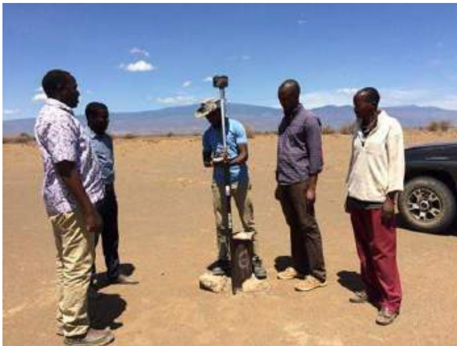
Figure 6.22. Photo showing DGPS survey on borehole number 6
